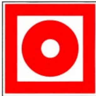
F08 Brandmelder (manuell)
